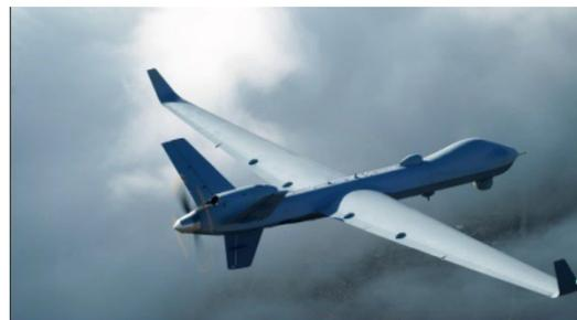
*MQ-9 Unmanned Aircraft System showcasing its Big Wing configuration.*
